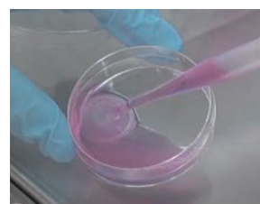
⑦ Tweezer the edge side of tiny hole (Not centered) where is on the side of the bottom, then take off the mesh.
