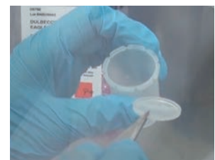
⑦ Tweezer the edge side of tiny hole (Not centered) where is on the side of the bottom, then take off the mesh.
