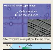
Easier to count because cells do not get stuck on the grid lines that are molded in the groove form.
