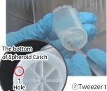
Tweezer the edge side of small hole (Not centered) where is on the side of the bottom, then take off the mesh.
