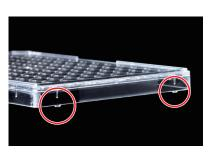
The lid design of the cover minimizes the contact with the surface of work space.
