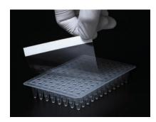
We use a newly developed optimized adhesive that changes its adhesion strength depending on the pressure applied when attaching the film. The more pressure you apply from above, the stronger the adhesion becomes, making it less likely for the film to peel off from the plate.
