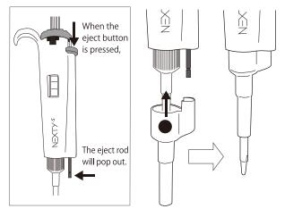
While pressing the eject button, align the eject rod that has popped out and press the new eject cone into place.
